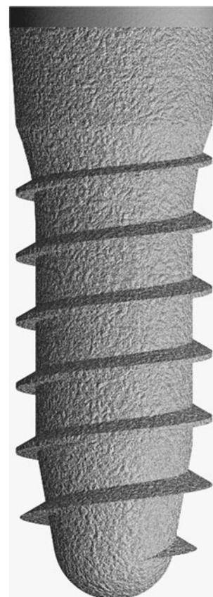
washing for 5 min in distilled water in a sonic bath [23–26]. The direct laser preparation provided an implant surface with a roughness surface that had an Ra value of 66.8, Rq value of 77.55, and Rz value of 358.3  $\mu\text{m}$ , respectively [23, 24] (Fig. 2).
